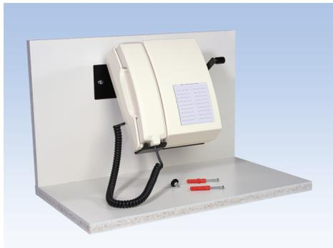
The telephone wall instrument is conceived as telephone, which can be operated independent from an external current supply (local battery operation / emergency operation). The ringing current is generated with the built-in crank inductor. The speaking current is supplied via 2 mono cells.
