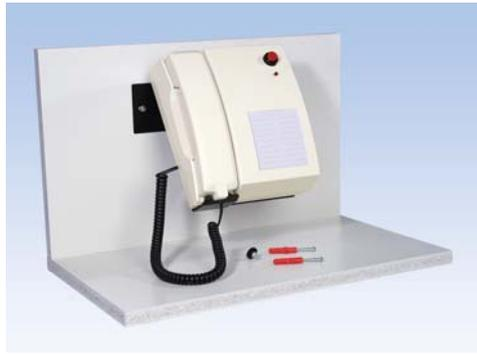
The telephone wall instrument is conceived as telephone, which can be operated by a 24 V current supply (central battery operation). The ringing signal is released by the push-button switch. The wall telephone is suitable for telephone transmissions over short distances. It is intended for stationary operation (fixed connection). The instrument is screwed onto a wall console.
