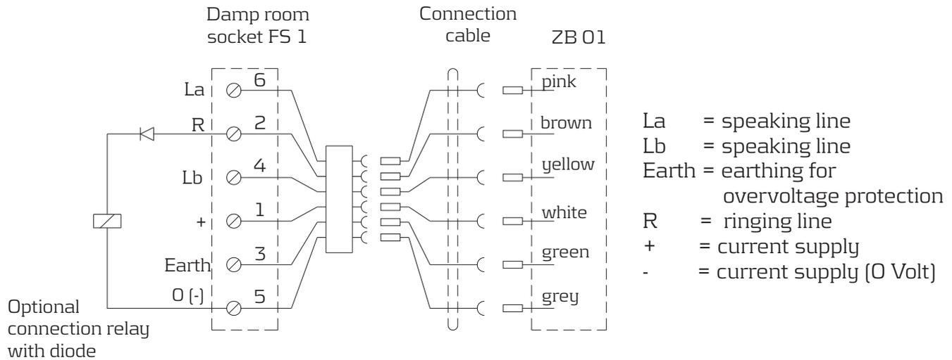
The use of the connection relays (2 x um, 1440 Ohm co. Schrack / type Siemens) is left to the user.
