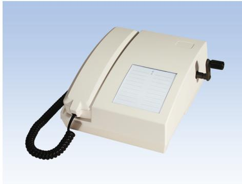
The telephone table instrument is conceived as telephone, which can be operated independent from an external current supply (local battery operation / emergency operation). The ringing current is generated with the integral crank inductor. The speaking current is supplied from 2 mono cells. The telephone table instrument is suitable for telephone transmission over long distances. It is intended for stationary operation (fixed connection).
