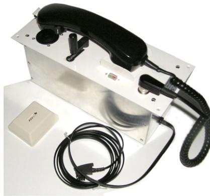
The telephone for installation is conceived as a telephone, which can be operated independent from an external current supply (local battery operation / emergency operation). The ringing current is generated with the integral crank inductor. The speaking current is supplied from 2 mono cells. The instrument is used for table, cabinet or door installation. The telephone is suitable for transmission over long distances. It is intended for stationary operation (fixed connection).
