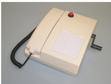
The telephone table instrument is conceived as a telephone, which can be operated independent from an external current supply (local battery operation / emergency operation) as well as by call remote power supply. The ringing current is generated with the integral crank inductor. The speaking current is supplied from 2 mono cells. The telephone table instrument is suitable for telephone transmissions over long distances. It is intended for stationary operation (fixed connection).
