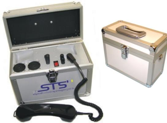
The telephone OB 06 can be operated independent from an external current supply (local battery operation / emergency operation). The ringing current is generated with the integral crank inductor. The speaking current is supplied from 3 mono cells. The telephone OB 06 is suitable for telephone transmissions over long distances. It is intended for use on construction sites and changing usage locations. The instrument can be integrated into an existing OB network.
